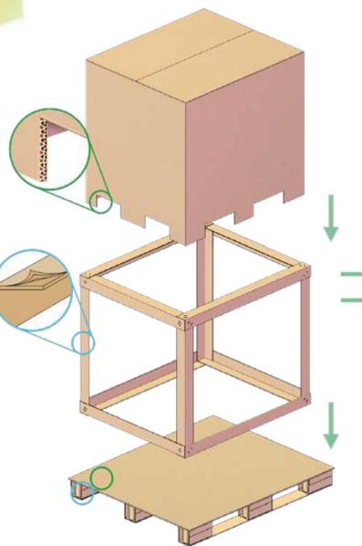
FrameBox is a combination of a Carton Board Pallet, FramePack corrugated board box and strapping.
